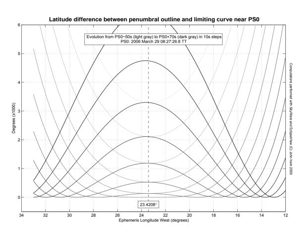
I have also generated an additional plot, included on the previous page, which attempts to show how the latitude difference evolves in time. Curves are shown at 10 second intervals from 50 seconds before PS0 to 70 seconds after. The longitude of PS0 is indicated by the central dotted line.
